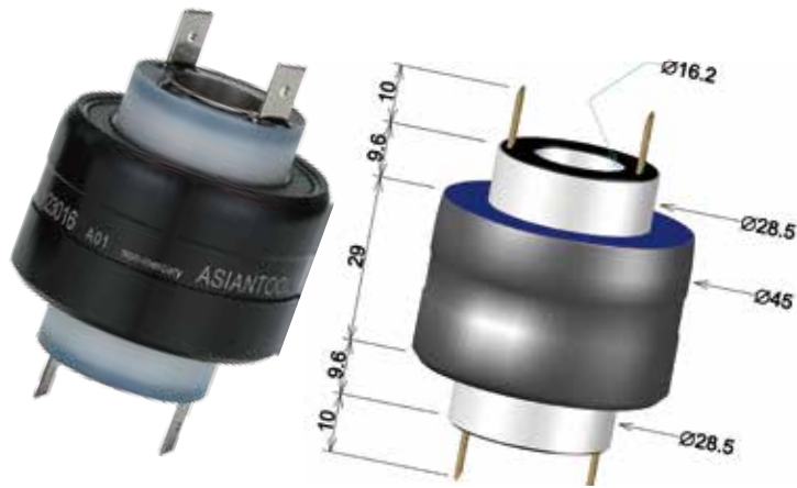
H23016 NM (non-mercury) 2poles/30A/AC250V Through-bore:16.2mm
